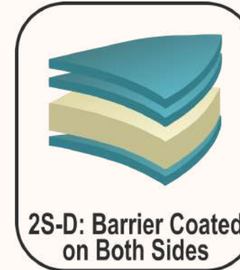
2S: Barrier Coated on Both Sides
